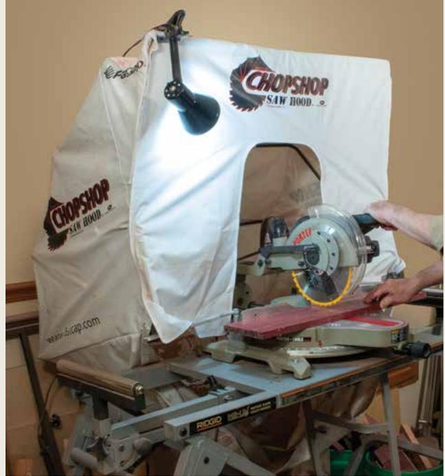
the floor. And the hood is waterproof, so you can also use it with a wet tile saw. Paired with a shop vacuum, this is a worthy investment for quality dust control at the miter saw. —Robert J. Settich
