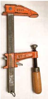
*I've been using a trick similar to the Bar Clamp Hold-Down tip (Dec/Jan 22), but less destructive to the clamp. I drill out the rivet at the end of the bar so I can remove the handle end. Slip the bar through the bench dog hole from below, then reinstall the handle above the table. I replace the rivet with a spring clip to keep the clamp parts together. Changing positions is a little slower, but clamping through the table means no chance of slipping.*
