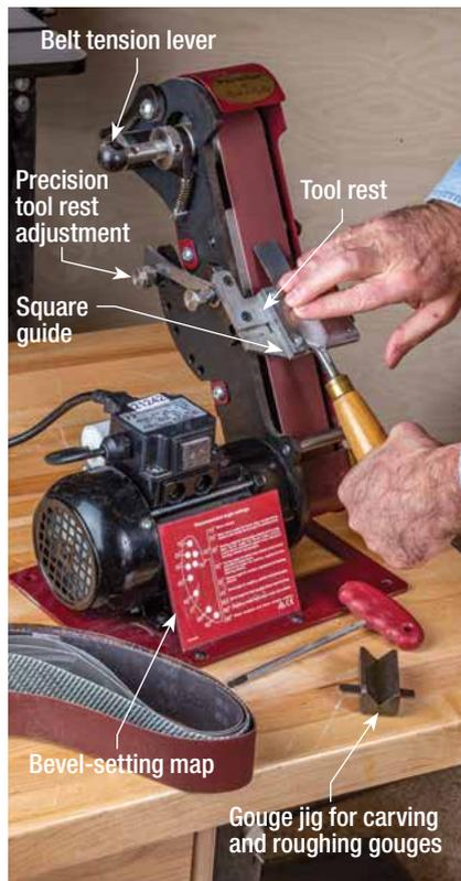
**Angle and abrade.** The ProEdge's tool rest is similar to a high-end rest for a bench grinder with the added benefit of a precise angle setting system. The only drawback is that it doesn't accommodate chisels with short blades.
