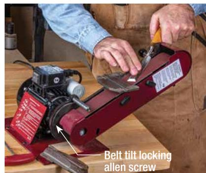
**Tilt and polish.** You'll need access to the backside of the machine when it's time to hone the back of your flat tools. Tilting the belt to a comfortable position requires loosening two Allen screws and then retightening to lock it in place.
