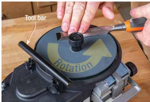
**Flatten topside.** The dead flat tempered glass plates faced with the right abrasive make short work of flattening the back of a new blade. A spare plate faced with the finest grit paper allows working the bevel below and the back above without stopping to flip or switch plates.
