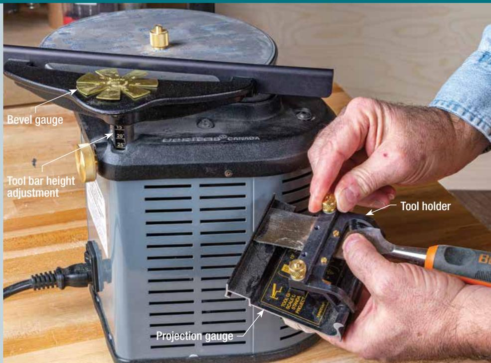
**Set the projection.** After adjusting the height of the tool bar to the desired bevel angle, set the projection. Clip the tool holder to the bar of the projection gauge, and slide the tool through the holder until its tip touches the gauge's flange. Tighten the holder knobs to lock the tool in place.
