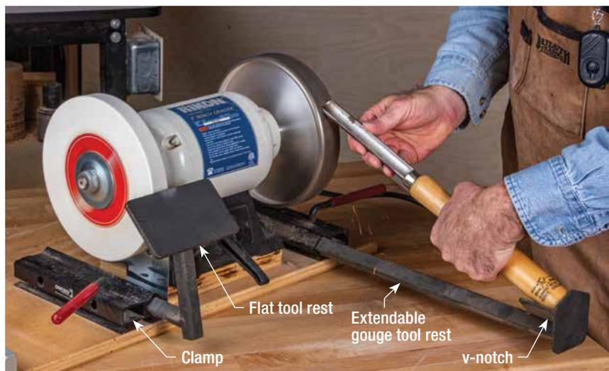
**Set and roll.** With the tool rest locked at a predetermined distance from the grinder, sharpening a gouge is a matter of dropping the handle in the v-notch and rolling it against the wheel as it spins. ■
