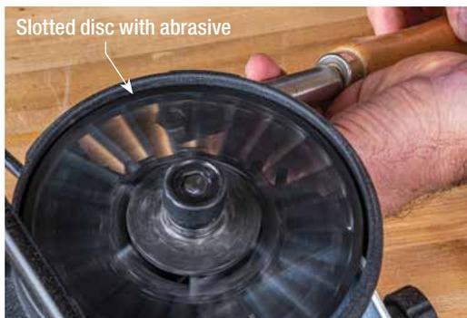
**Eyeballing underneath.** Swap the glass plate for the plastic slotted one with its matching abrasive paper, and you'll be able to see through the disc as it spins. This allows you to sharpen non-square tools such as skew chisels on the ramp or large lathe tools to the side by eyeballing how they contact the abrasive.
