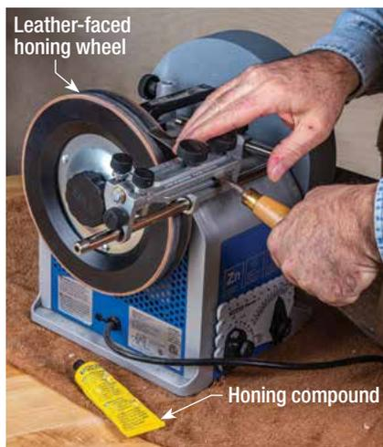
**Hone to perfection.** After charging the leather with the provided honing compound, reposition the tool bar and keep the tool in the holder as you hone the bevel. Polishing the back is done freehand.
