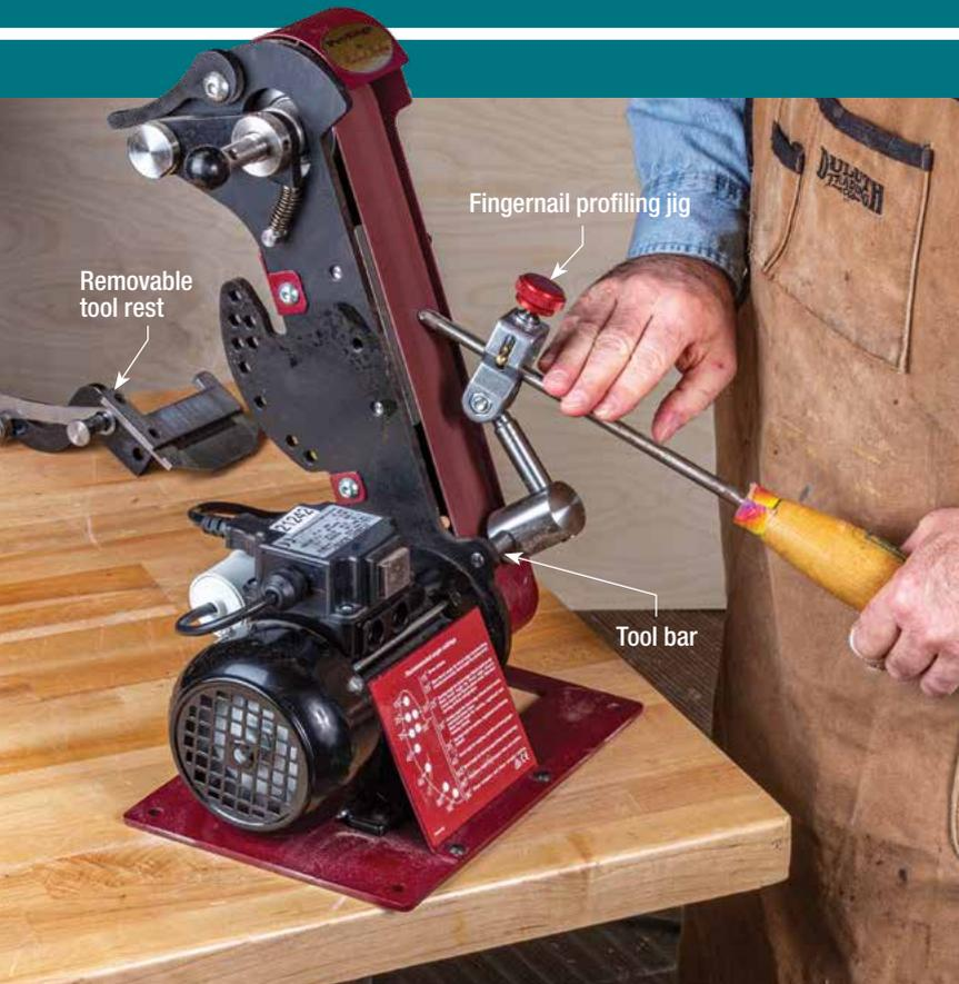
**Pivot and grind.** The fingernail profiling jig comes with the machine and allows you to perfectly reproduce the standard grind on the end of a bowl gouge by pivoting the tool as you roll it against the belt.
