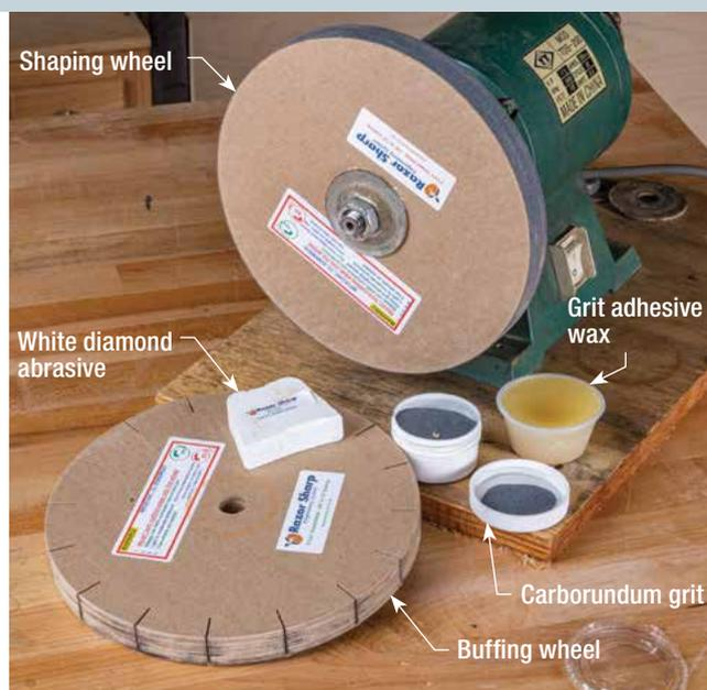
**Paper wheels.** Razor Sharp's system is based on two laminated paper wheels that provide a firm surface and hold up surprisingly well. The rim of one gets charged with abrasive grit for shaping; the rim of the other, with white diamond buffing compound.
