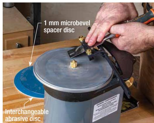
**Freehand finesse.** To set the bevel when sharpening gouges, rest the tool on the bar using your finger as a stop to determine the projection, eyeballing the bevels contact with the abrasive. Gently roll the tool with your opposite hand.
