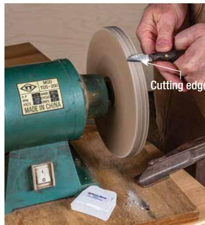
**Freehand buffing.** To avoid damaging the paper wheels, hold your tools cutting-edge down. No gauge or tool rest required; simply grind and buff the bevels by feel.
