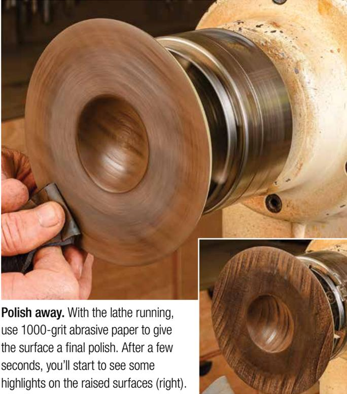
**Polish away.** With the lathe running, use 1000-grit abrasive paper to give the surface a final polish. After a few seconds, you'll start to see some highlights on the raised surfaces (right).
