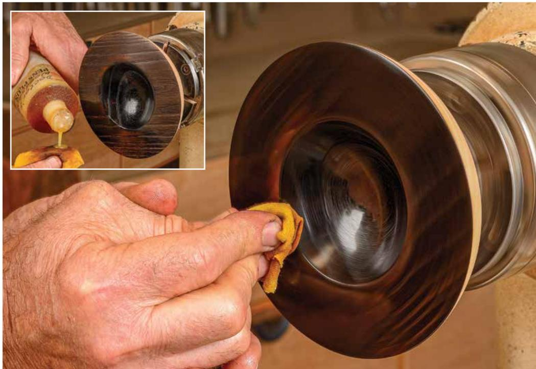
**Seal the surface.** Dab the friction polish onto the surface with the lathe stopped (inset). Because the back of the bowl isn't necessarily ready for finish, you don't want to risk contaminating it as you might were the lathe spinning. Once the surface is coated, run the lathe to buff the finish and force it into the surface.
