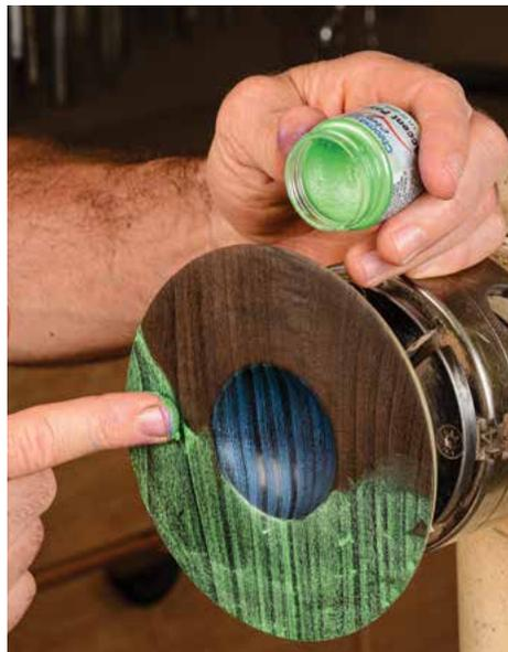
**Add the second color.** Rub in the next color, being careful at the edges to keep the colors separate. Fortunately, you can readily remove the paste from previously buffed areas as long as you haven't pushed it hard into the surface.
