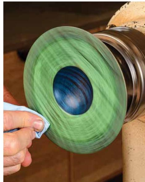
**Buff, buff, buff.** With the lathe spinning at about 1800 RPM, buff the surface with a rag or paper towel. This is where you'll be creating that beautiful mottled surface effect and remove any excess paste.
