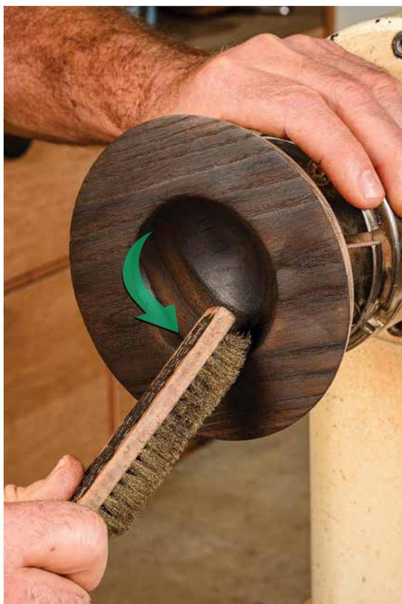
**Follow the contour.** Keep following the grain as you brush the inside of the bowl, this may require a kind of twisting stroke.
