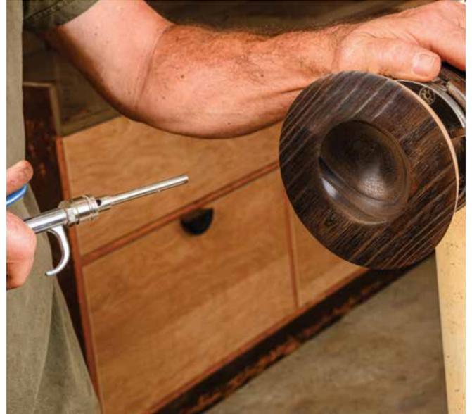
**The blow off.** After sanding, blow off the surface thoroughly to clean the dust out of the pores. You'll see the surface transform from a frosted white to a clean brown.
