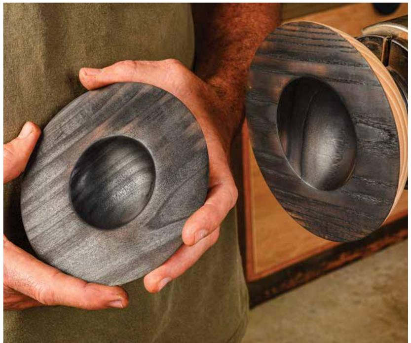
**Texture to the forefront.** A consistently burned surface creates pronounced grain texture even in mild-grained species such as poplar (left). In a coarser-grained wood such as ash (right) the texture is even more striking. Note that both of these bowls were dead smooth before torching.
