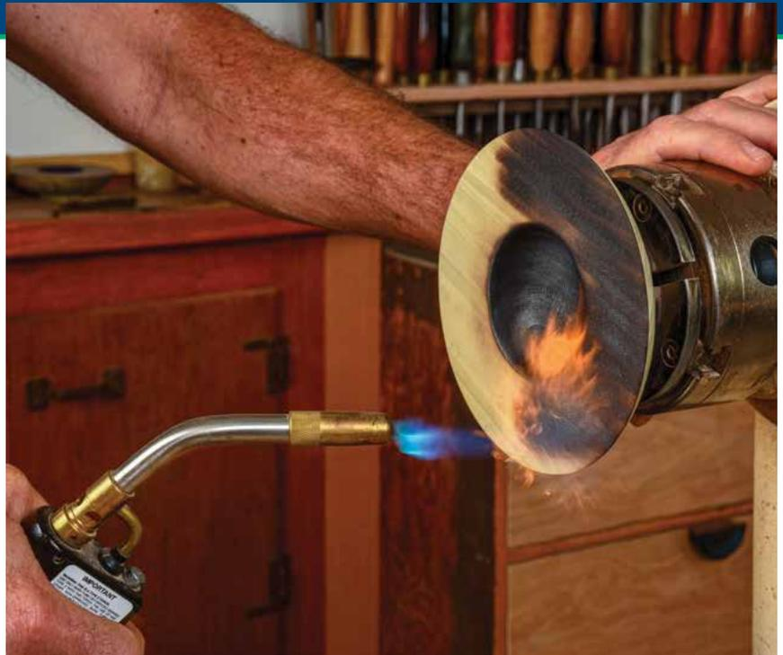
**Inside out.** Start with the inside recess and work your way outward. Quickly “paint” the surface with the flame, trying to achieve a consistent overall scorch. Keep the torch moving and try not to let the wood actually start to flare up. Be particularly careful at the edges as they will check if they get too hot.
