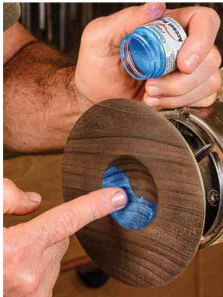
**Rub it in.** I find it works best to rub in the paste with my finger. This way I can really work it well into the pores. It wipes and washes off readily afterward so I don't look like a smurf the rest of the day. Power-buff to polish and set the color.
