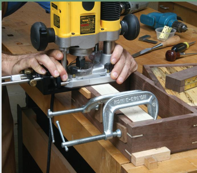
**CLAMP A SHORT BOARD** to the box wall to support the base of the router. Use an edge guide to rout the long rear wall of the mortise.
