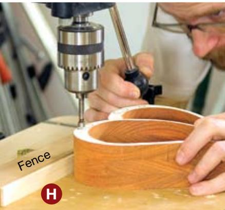
Set up your drill-press fence to align the hinge mortise centerpoints. This is crucial for smooth hinge operation.
