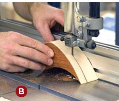
Use a fence on your bandsaw to help stabilize the stock when resawing it.
