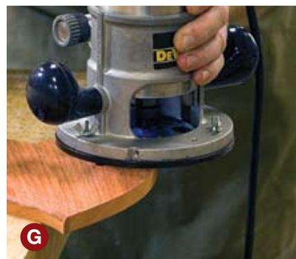
**G** Use a router to round over the top edge of the base. A laminate trimmer would be even easier to handle for this task.
