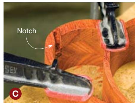
Chisel a notch on the bottom edge to house the spring wire that turns the music box movement on and off.
