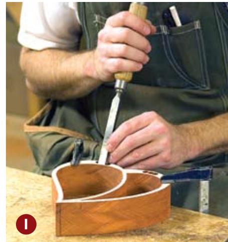
Clean up the hinge mortises with a chisel so that the hinge edge fits closely and the hinge sits flush to the surrounding wood.
