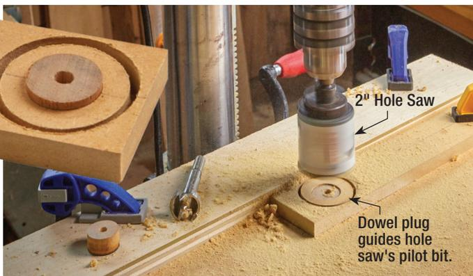
**Step 2:** Without moving the table or workpiece, replace the 1" Forstner with a hole saw. A 2"-diameter hole saw is shown here, but the actual size isn't important as long as the diameter of the cutout is larger than 1½". (*Note: Without proper guidance, hole saws tend to wobble when making a cut. To keep the saw on track, cut a short piece from a 1"-diameter dowel, and use it to temporarily stop the hole in your MDF strip.*)
