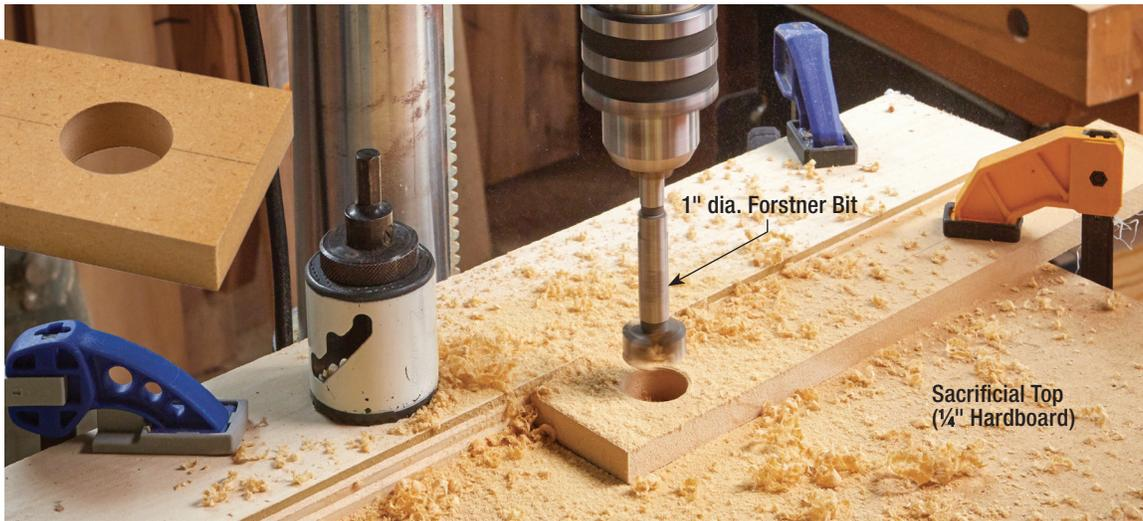
**Step 1:** Secure a strip of ½" MDF (about 2¼" wide and approximately 10" long) to your drill press table. Drill a 1"-diameter hole, as shown.
