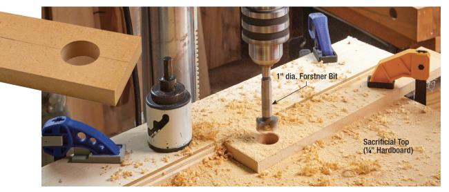
Step 1: Secure a strip of ½" MDF (about 2¼" wide and approximately 10" long) to your drill press table. Drill a 1"-diameter hole, as shown.
