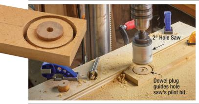
**Step 2:** Without moving the table or workpiece, replace the 1" Forstner with a hole saw. A 2"-diameter hole saw is shown here, but the actual size isn't important as long as the diameter of the cutout is larger than 1½".) (*Note: Without proper guidance, hole saws tend to wobble when making a cut. To keep the saw on track, cut a short piece from a 1"-diameter dowel, and use it to temporarily stop the hole in your MDF strip.*)
