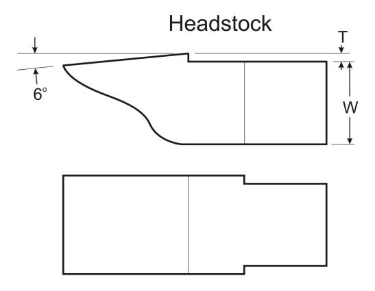
Note: T= soundboard thickness W= side piece width
