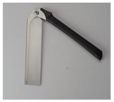
**Protected precision.** The fine, razor-sharp teeth on a Japanese saw are easily damaged. So if you want a dozuki saw that can travel well in a tool tote, this folding Silky Saws WOODBOY is just the ticket. The 240mm blade has 27 TPI. The rubber-covered handle is comfortable to hold, and is slotted on one side to protect the teeth when the saw is folded shut.
