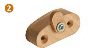
**Dovetail Saws** (1"-thick bandsawn shape to match handle openings; turn button)
