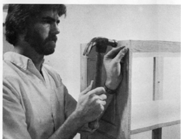
8. NAIL AND GLUE COMPLETED SIDE PANELS TO O,P,Q AND FRONT FACE FRAME.
