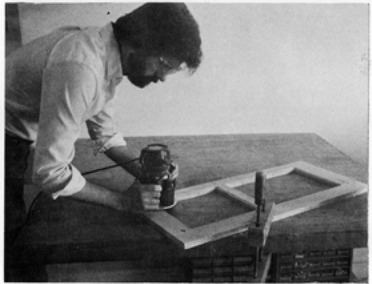
5. ROUT BACKSIDE OPENINGS OF SIDE PANELS AND BACKSIDE OF FRONT DOOR FRAMES FOR INSERTION OF 1/8" PLYWOOD.
